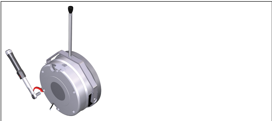
Fig. 9 Mounting the stator to the end shield
